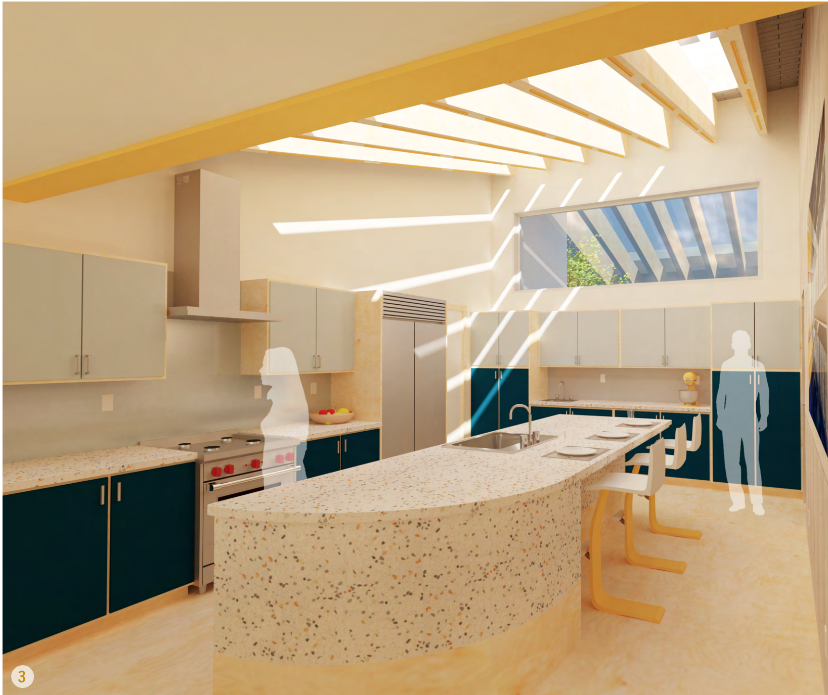
Kitchen depicting partial overlaid cabinetry, terrazzo counters and an asymmetrical island. The backsplash features glass with a custom-painted reverse surface. Steel painted beam in yellow safflower visually divides the kitchen and dining spaces.
